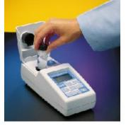
With a measurement range of 0 to 1000 NTU and a resolution of 0.01 NTU, the 2100P is ideal for regulatory monitoring, process control or field studies.
