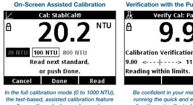
walks you through clear and easy steps, and verifies the accuracy of your calibration automatically. This on-screen assistance eliminates the need for a manual and provides assurance that your calibration is complete and valid.
