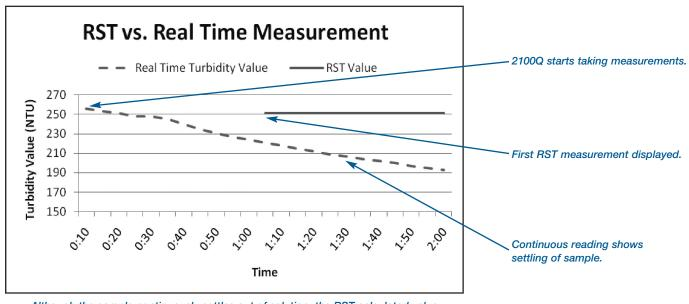
Although the sample continuously settles out of solution, the RST calculated value does not change. No more guessing and no more replicate runs -you get the right answer every time.
