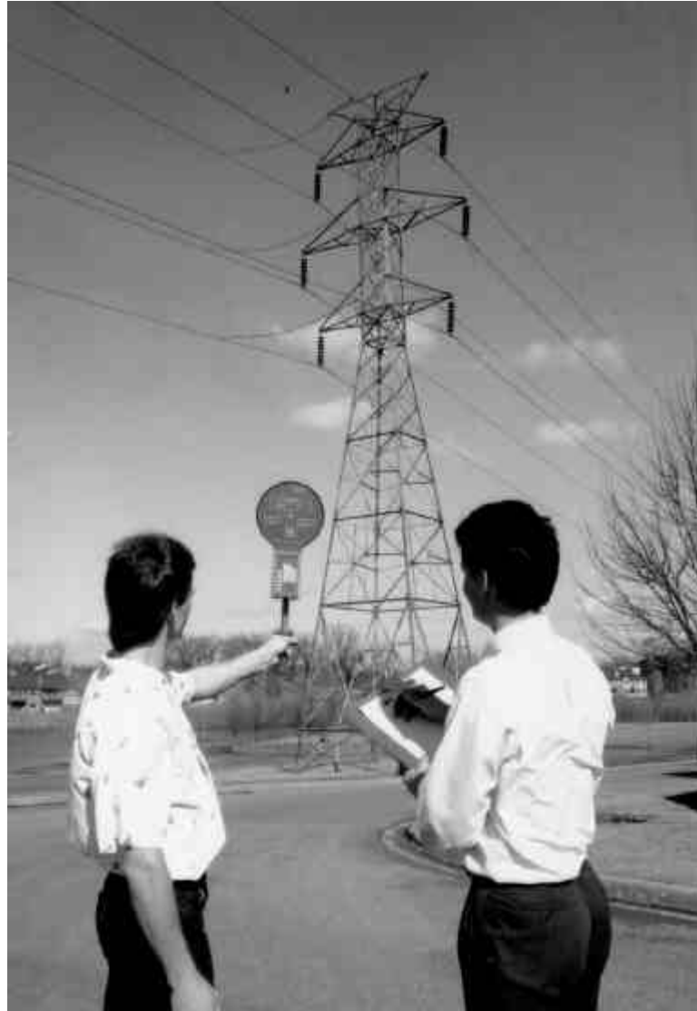
Figure 1-1 HI-3604 ELF Field Strength Measurement System
