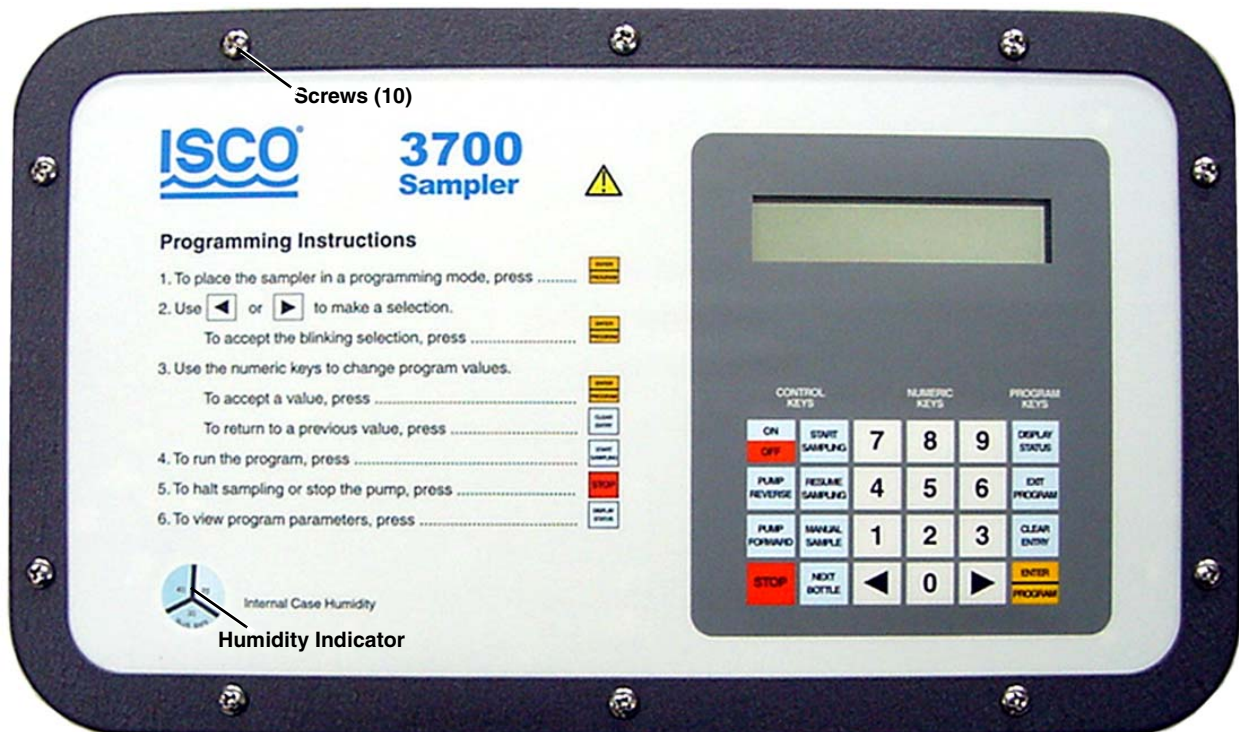
Figure 5-4 Location of 10 Screws on Control Box Lid
