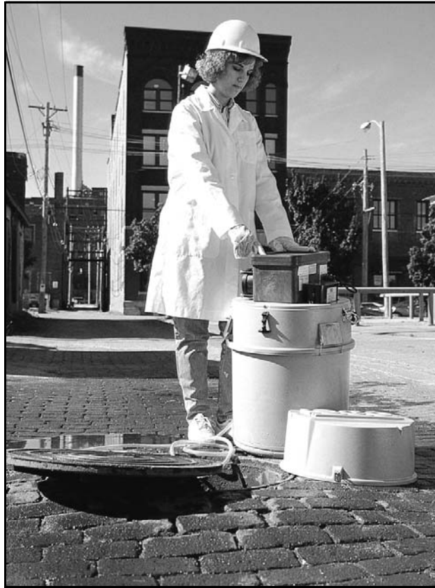
Figure 2-6 Placement of the Sampler Adjacent to Manhole
