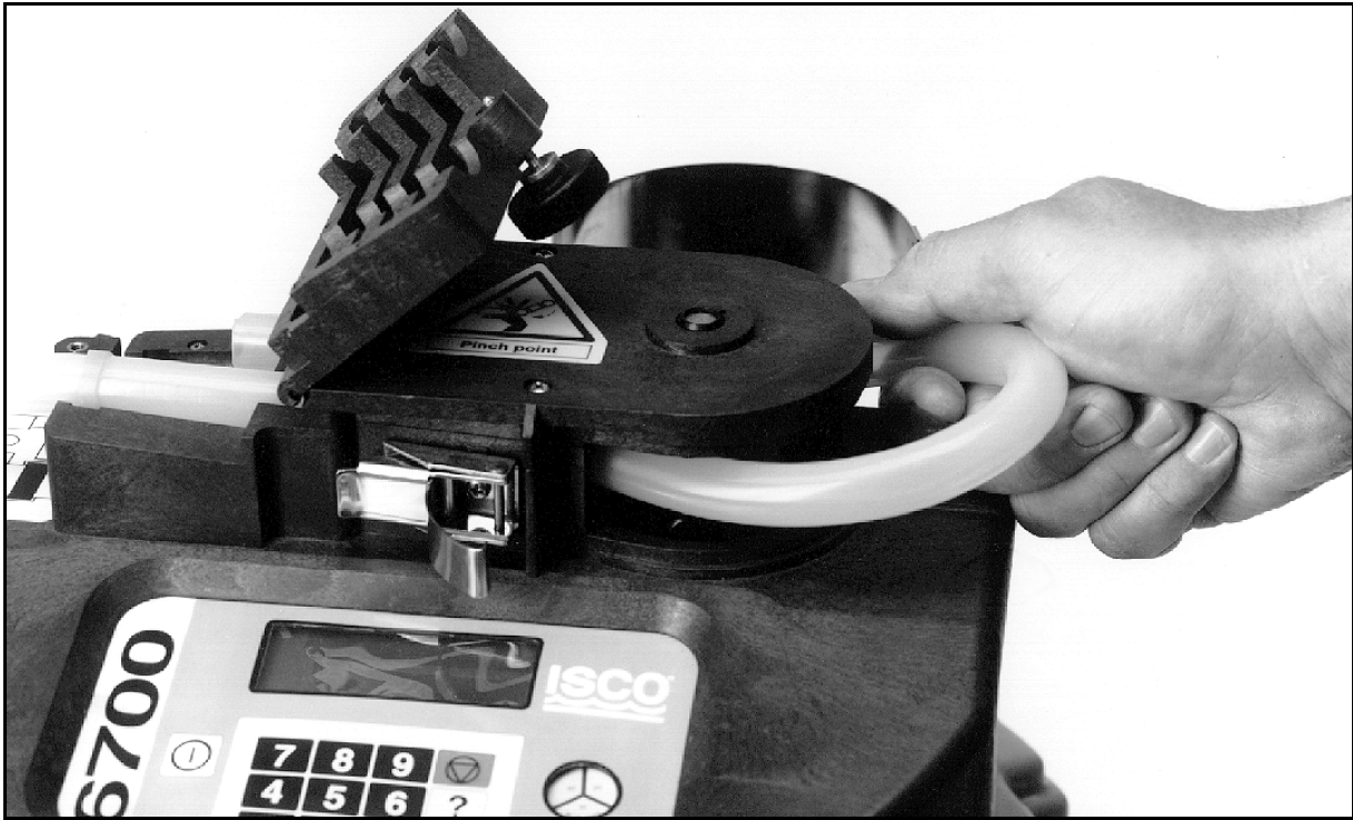
Figure 17 Removing and Replacing the Pump Tube
