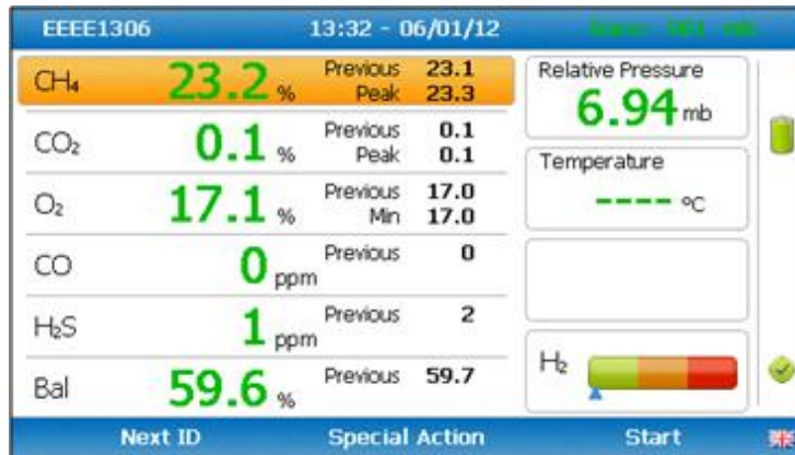
Figure 29—Analyzer in GA Mode—Main Gas Reading Screen
