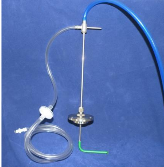
Figure 30—Example of a Pitot Tube
