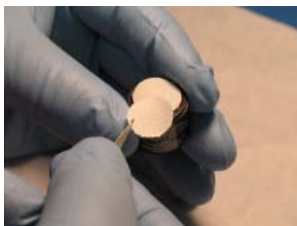
Figure 7-14. Placing the Filter Media
