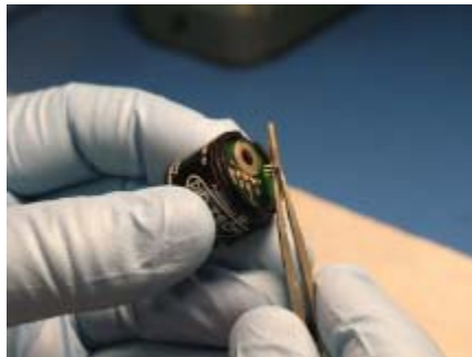
Figure 7–12. Installing the Cell Assembly
